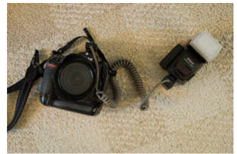
Using cable to get the flash off the camera.
